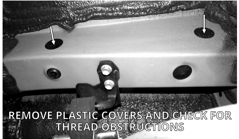
FIGURE A1: VIEW OF THE REAR FRAME UNDER THE VEHICLE
