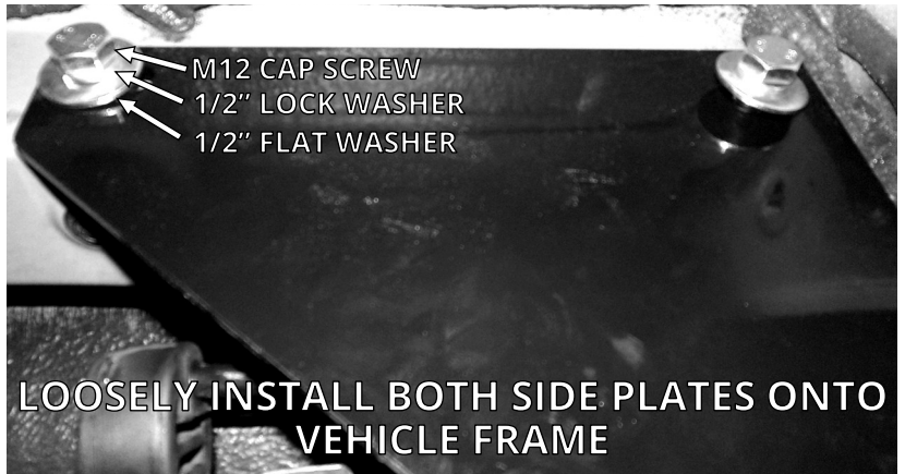
FIGURE B1: SIDE PLATE INSTALLATION
