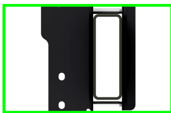
FIGURE C6: View showing a correctly tightened inside clamp.
