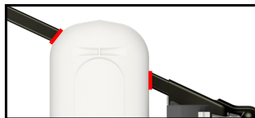
FIGURE C1: Top of A-frame with propane tank cover.
