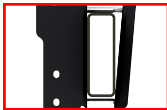
FIGURE C7: View showing an incorrectly tightened inside clamp.
