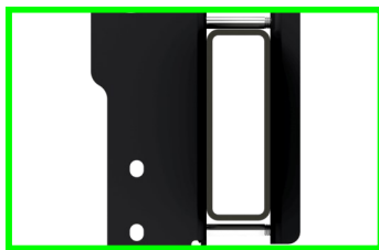
FIGURE C6: View showing a correctly tightened inside clamp.
