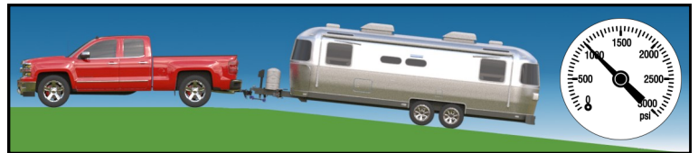
FIGURE L5: Truck and trailer angled down (lower pressure)
