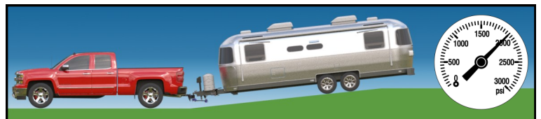
FIGURE L4: Truck and trailer angled up (higher pressure)
