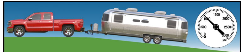
FIGURE L5: Truck and trailer angled down (lower pressure)
